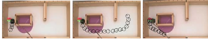
Fig. 2. In the experiments, a trial ended either after a collision or a maximum of 40 steps. The generated behavior shows that only the explicitly planning system ( middle ) was able to realize a successful obstacle avoidance considering the physical limitations of the non-holonom robot with a very limited action space. After the very first detection of a curve or obstacle, this system began to move to the left (as second selected action) and pursued that movement until the turn was negotiated. In contrast, the reactive system ( left ) chose to drive straight forward until almost hitting the wall. Only directly in front of the wall it chose to turn right, thus unable to avoid a collision. The Q-learning system ( right ) initiated also an early turn to the left and continued until the turn was negotiated. Subsequently, the action 'go straight' was repeatedly chosen, because the visual situation in the middle of the floor is represented by the same Fuzzy ART node as the floor situation near the wall. Only in the situation directly in front of the wall, another Fuzzy ART node was activated and a turn initiated. Like Q-learning, our reactive approach also learned the action 'go straight' for the floor situation, but by means of internal simulation, it chose mostly turns.
