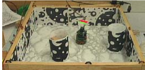
Fig. 1. Scenario used for our experiments with the mobile robot KHEPERA equipped with an omnidirectional camera.
