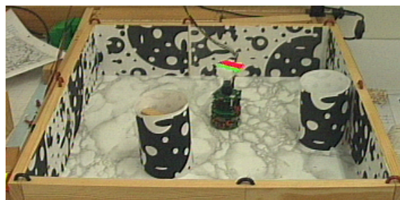
Figure 1: View of the used environment with the robot KHEPERA, equipped with an omni-directional camera.
