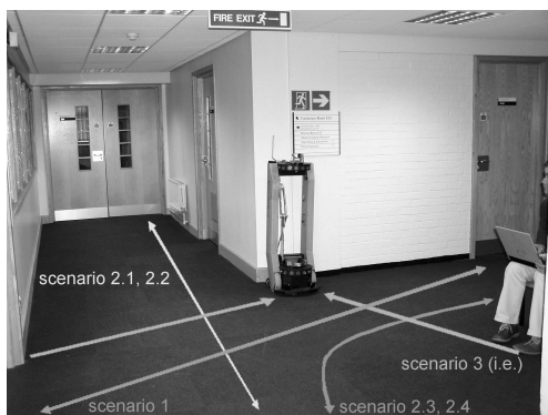
Fig. 3. Environment of the first experiment. The movements of the three scenarios are shown by the arrows. Scenario 1 corresponds to the subject moving from "right to left" and "left to right" in front of the robot. Scenario 2.1 and 2.2 have the subject moving past the robot on its right side from front to back and visa versa. Scenario 2.3 has the subject moving along a curved path from the robot's front to the passage at the robot's left. Scenario 2.4 is the same but with the subject moving in the opposite direction. Scenario 3 corresponds to the subject moving "forward" in a straight line from anywhere within a semi-circle ahead of the robot, stopping in front of the robot.
