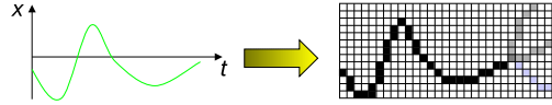
Fig. 1. Motion Trajectories are transferred into a grid representation. A grid cell is set to 1 if it is in the path of the trajectory and set to zero otherwise. During the prediction phase multiple hypotheses can be gained by superimposing several basis primitives. This is indicated with the gray trajectories on the right side of the grid.
