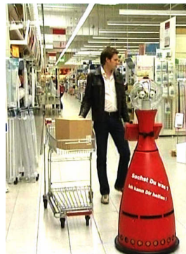
Fig. 1. Interactive mobile shopping assistant TOOMAS guiding a customer together with his shopping trolley to the location of the product of his choice in a typical home improvement store.
