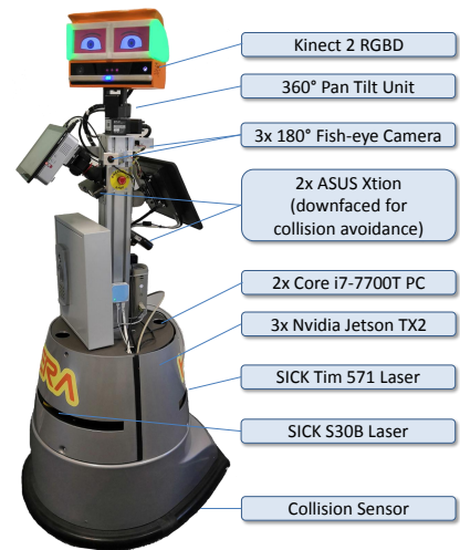
Fig. 2: Used robot platform with its sensors and processing hardware.
