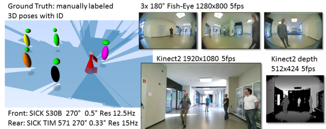
Fig. 1: A snapshot from our dataset with all the data channels recorded. Colored blobs are the ground truth labels, while the green blobs are the results of our tracker focusing on the people's heads
