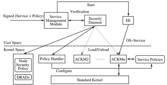
Fig. 1. The Architecture of the Access Control Mechanism
