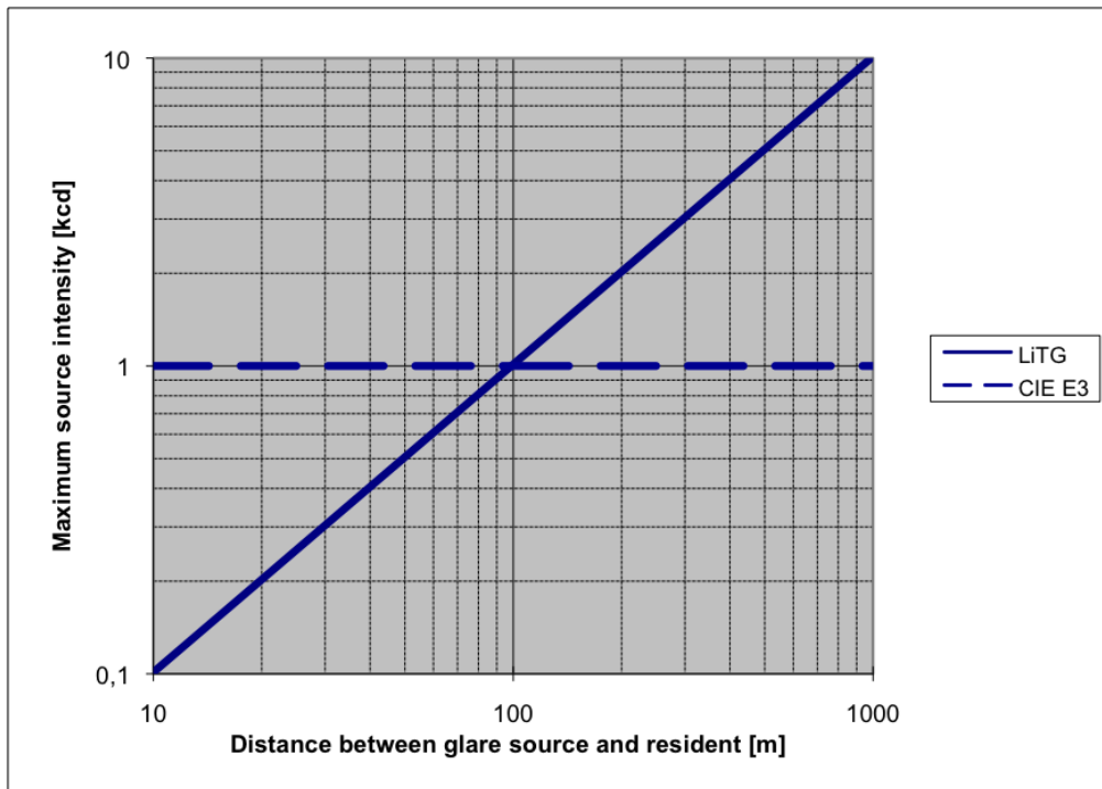
Figure 3. Comparison between the CIE and LiTG method.
