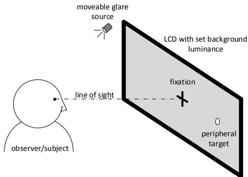
Fig.: Initial set-up of the direct compensation method for a peripheral target position
