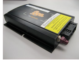
Fig. 4: On-Board Unit with OBD Interface and GSM/GPRS Uplink
